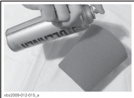
TYPICAL - SPRAY FOAM ELEMENT INSIDE AND OUT
