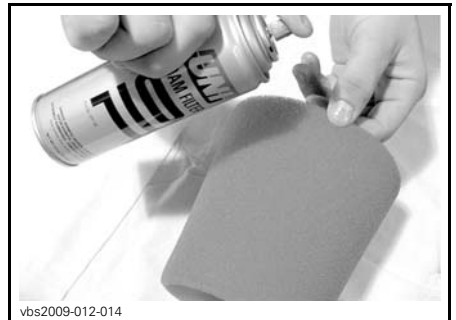
TYPICAL - OIL THE FOAM FILTER
