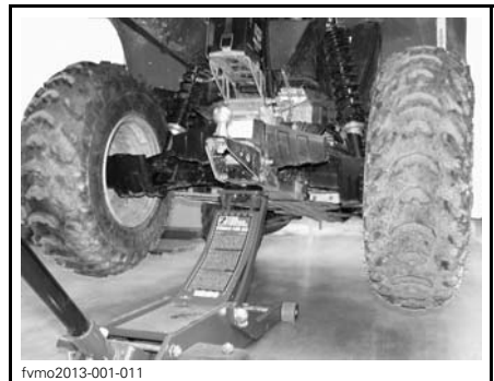
TYPICAL — REAR LIFTING POINT
