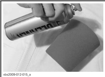
TYPICAL - SPRAY THE FOAM FILTER
