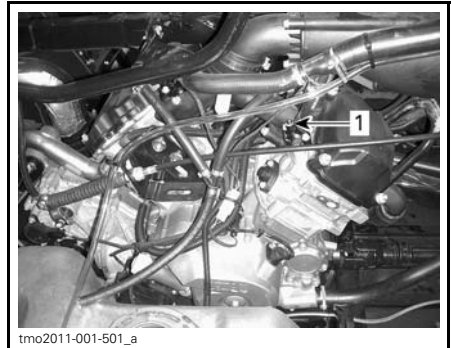
1. Front cylinder bleed screw
