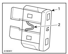
**TYPICAL** 1. Fuse 2. Check if melted
