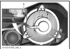
LOW BEAM 1. Adjustment knobs
