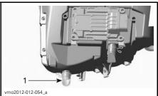
TYPICAL 1. Air filter housing drain reservoir
