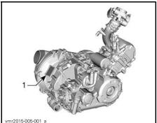
BACK OF 450 ENGINE 1. EIN (Engine Identification Number)
