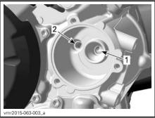
Inlet bore from the oil pump to the oil filter
