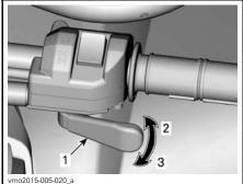
**TYPICAL** 1. Throttle lever 2. To accelerate
