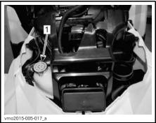
1. Engine coolant reservoir cap
