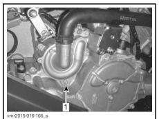
TYPICAL - SOME PARTS REMOVED FOR CLARITY 1. Coolant drain plug
