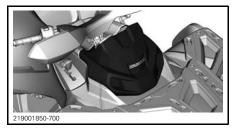
Remove engine coolant reservoir cap. With vehicle on a level surface, liquid should be between MIN. and MAX. level marks of coolant reservoir.
