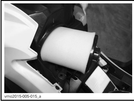
AIR FILTER REMOVAL
