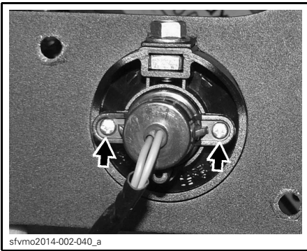
sfvmo2014-002-040_a UNSCREW SECURING SCREWS FROM REAR TURN SIGNAL BULB
