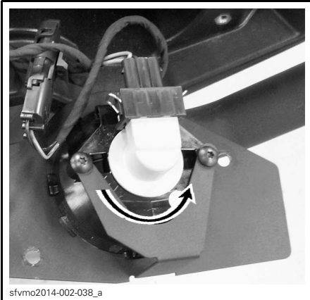
sfvmo2014-002-038_a TYPICAL: ROTATE BULB COUNTERCLOCKWISE
