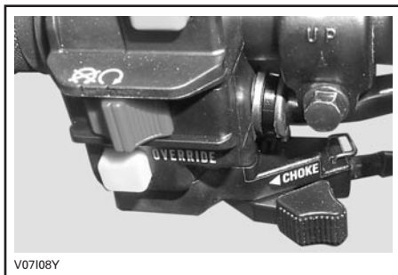
CHOKE LEVER IN THE OFF POSITION
