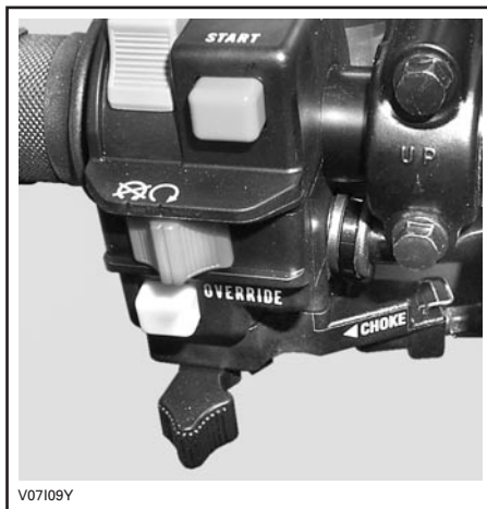
CHOKE LEVER IN THE FULL CHOKE POSITION
