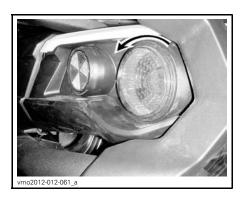
Pull tail light out of its location. Unplug connector from bulb.
