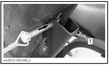
1. Bent plate of gun boot support
