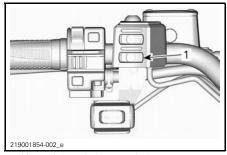
1. Heated throttle lever switch
