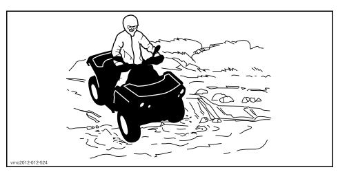
Wet brakes will affect the braking ability of your vehicle. Make sure you dry the brakes by applying them several times after the vehicle leaves the water, mud or snow. Allow greater distance for braking.
