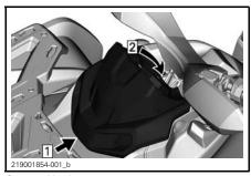
Step 1: Hook Step 2: Engage retaining tab
