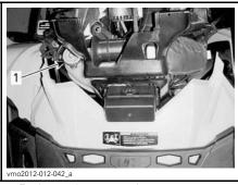
1. Engine coolant reservoir cap
