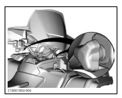
To install, insert the windshield arms into their supports, then hand tighten the knobs.
