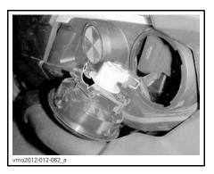
Remove bulb socket from taillight. Installation is the reverse of the removal procedure.
