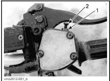
1. Lock nut 2. Speed limiter screw
