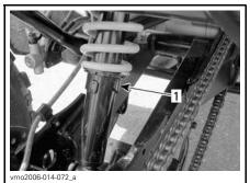
**REAR SUSPENSION** 1. Preload cam
