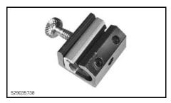
Insert the needle of spray can in the cable luber hole.
