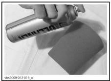
TYPICAL - SPRAY FOAM ELEMENT INSIDE AND OUT
