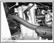
*LH SIDE OF ENGINE* 1. Air injection valve
