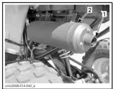
TYPICAL 1. Remove muffler end
