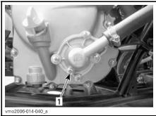
1. Cooling system drain plug
