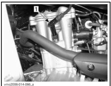
LH SIDE OF ENGINE 1. Spark plug
