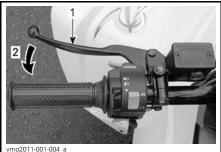
TYPICAL 1. Brake lever 2. To apply brake
