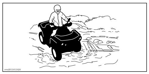
Wet brakes will affect the braking ability of your vehicle. Make sure you dry the brakes by applying them several times after the vehicle leaves the water, mud or snow.
