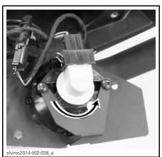
TYPICAL: ROTATE BULB COUNTERCLOCKWISE
