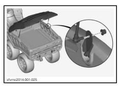
3. Remove pins from hinges both sides.
