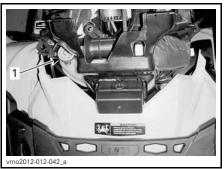
1. Engine coolant reservoir cap
