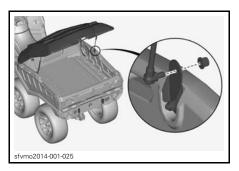
9. Install the shock's top end by screwing it into place.
