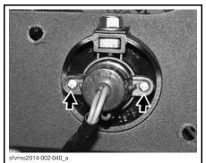
UNSCREW SECURING SCREWS FROM REAR TURN SIGNAL BULB
