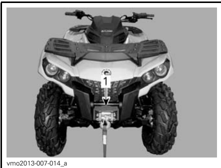
1. Front tie-down point location
