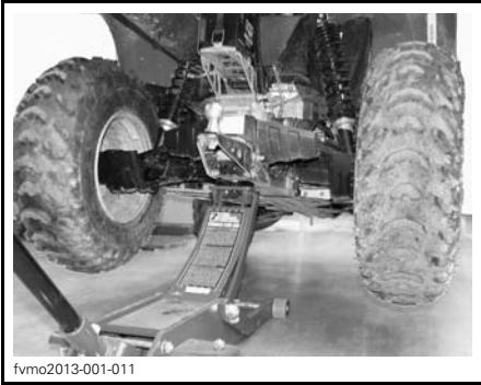
TYPICAL — BACK UP POINT LOCATION
