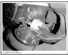
ROTATE BULB COUNTERCLOCKWISE
