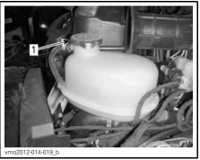
1. Engine coolant reservoir cap
