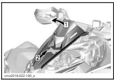
Step 1: Pull upwards Step 2: Pull rearwards
