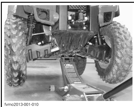
TYPICAL — FRONT UP POINT LOCATION
