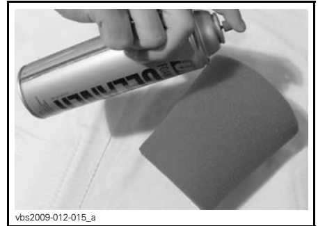
TYPICAL - SPRAY THE FOAM FILTER
