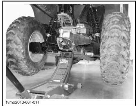
TYPICAL — BACK UP POINT LOCATION
