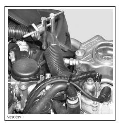
Fill the radiator until the coolant comes out by the thermostat housing hole. Install the bleeding screw then remove the hose pincher.
