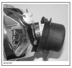
Unlock the bulb socket.
