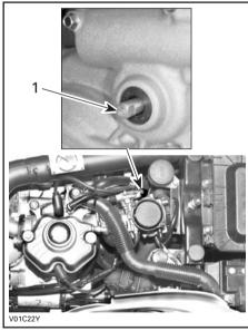
Emergency shifter shaft. Insert special tool here
