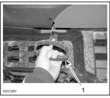
Grasp manual starter handle firmly and crank engine
