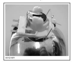
Install the protective rubber sleeve and connect the headlamp connector.
