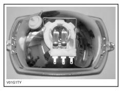
Remove the socket snap. Open the both side of socket snap.
