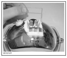
Push bulb in and hold while turning counterclockwise to release.
