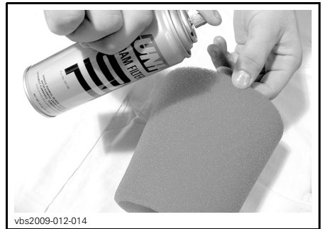
TYPICAL - OIL THE FOAM FILTER
