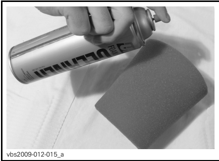
TYPICAL - SPRAY THE FOAM FILTER
