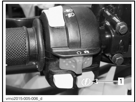
TYPICAL 1. Engine start button
