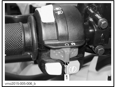
1. Emergency engine stop switch
