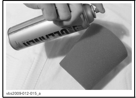
TYPICAL - SPRAY THE FOAM FILTER
