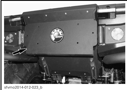
1. Rear storage compartment hatch
