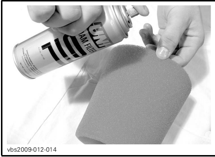
TYPICAL - OIL THE FOAM FILTER
