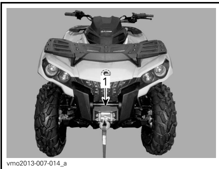
1. Front tie-down point location
