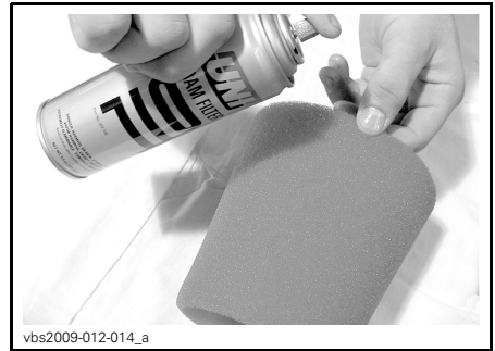
TYPICAL - OIL THE FOAM FILTER ELEMENT
