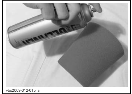
TYPICAL - SPRAY FOAM ELEMENT INSIDE AND OUT
