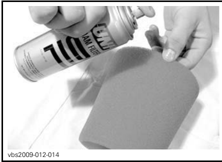
TYPICAL - OIL THE FOAM FILTER
