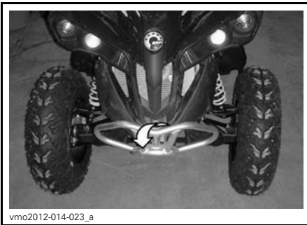
TYPICAL - FRONT TIE-DOWN POINT LOCATION
