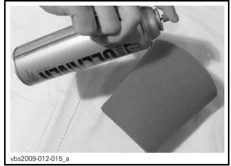
TYPICAL - SPRAY THE FOAM FILTER
