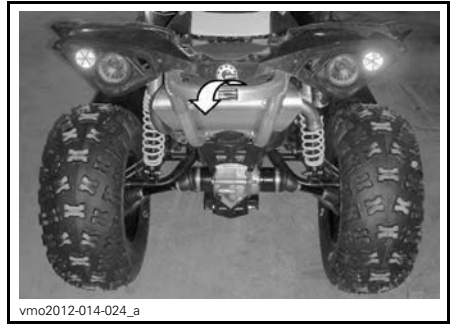
TYPICAL - REAR TIE-DOWN POINT LOCATION
