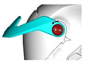
**3.** If helmet is equipped with a peak. Pull perpendicularly on the side of the peak as shown.
