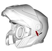
2. Insert the sun visor between helmet inner and outer shell and fit it on to the locating pegs on both sides.
