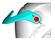
**2.** If the helmet is equipped with a peak, remove the peak screw by turning the external part a quarter turn counterclockwise.
