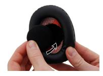
**A.6.** Reinstall the NCS into the helmet, making sure the openings are at the base of the helmet and the speaker cable is pointing toward the back of the helmet.
