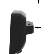
The VIBE UNIVERSAL will be in pairing mode at first start. To exit pairing mode, press the center button once.
