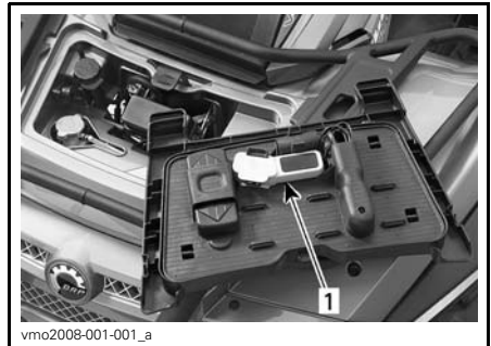
FRONT SERVICE COMPARTMENT 1. Winch remote control
