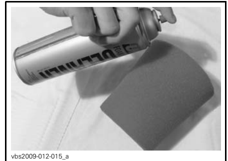
TYPICAL - SPRAY THE FOAM ELEMENT
