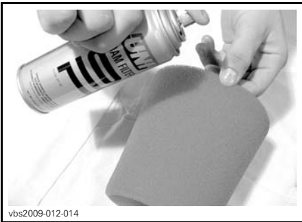
TYPICAL - OIL THE FOAM FILTER ELEMENT
