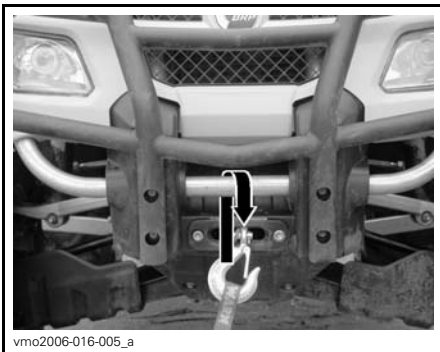
TYPICAL — FRONT TIE-DOWN POINT LOCATION
