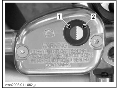
TYPICAL 1. Proper fluid level 2. Low fluid level
