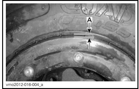
A. Gap (must be equal all around the wheel)
