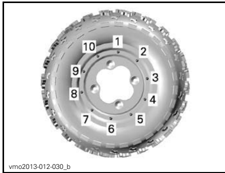
10-BOLT BEADLOCK WHEELS — FINAL STEP TIGHTENING SEQUENCE
