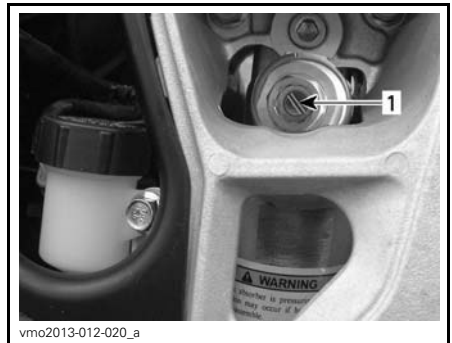
TYPICAL - DS 450/DS 450 X xc 1. Low speed compression adjuster (flat screwdriver)
