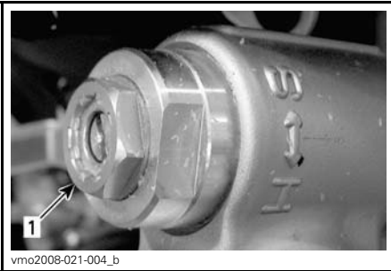
1. High speed compression adjuster (17 mm wrench)
