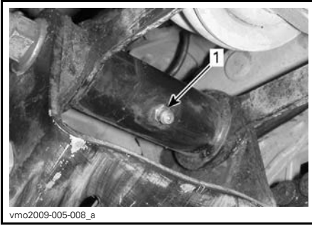
REAR PIVOT ARM 1. Grease fitting
