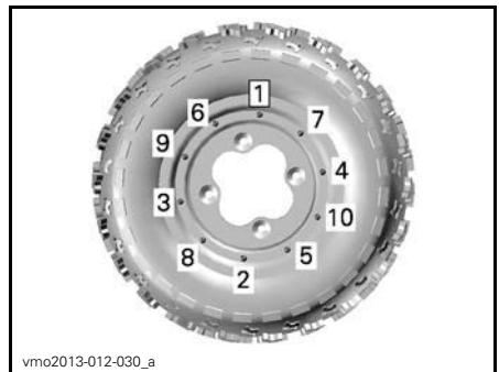
10-BOLT BEADLOCK WHEELS — FIRST AND SECOND STEPS TIGHTENING SEQUENCE
