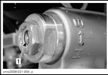
1. Low speed compression adjuster (flat screwdriver)
