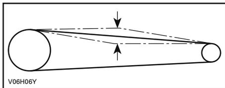
**FLÈCHE DE LA CHAÎNE D'ENTRAÎNEMENT ENTRE 15 MM ET 25 MM**
