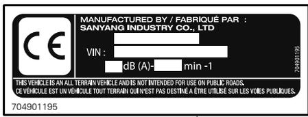
EMPLACEMENT: TUBE INFÉRIEUR AVANT DROIT DU CHÂSSIS
