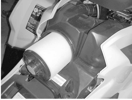
AIR FILTER REMOVAL
