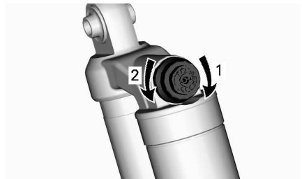
COMPRESSION DAMPING - TOP OF SHOCK ABSORBER
