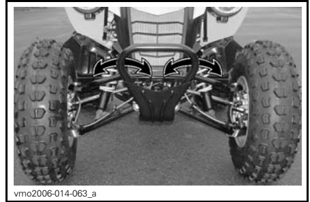
TYPICAL – FRONT BUMPER STRAP LOCATIONS
