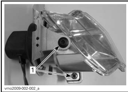
1. Screws to be loosened
