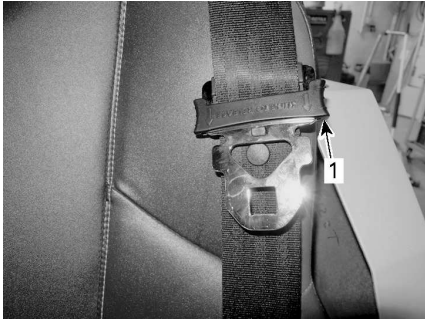
TYPICAL - LOCKED POSITION
