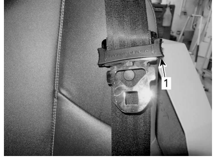
TYPICAL - LOCKED POSITION
