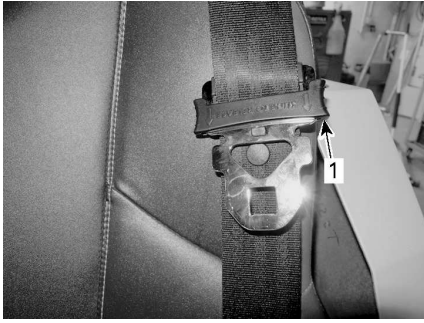
TYPICAL - LOCKED POSITION
