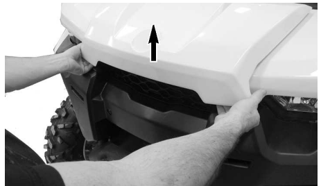
LIFTING FRONT SERVICE COVER EDGE.
