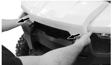
PULLING ON FRONT SERVICE COVER EDGE.
