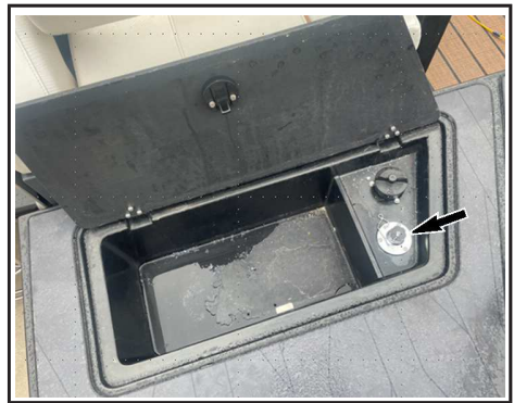
FLUSHING PORT — TYPICAL
