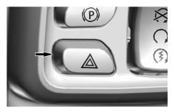
Push the button to turn ON the hazard warning lights.
