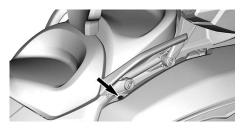
To activate or turn OFF the heating grip, press the button.
