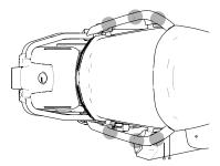
DIFFERENT GRIPPING POSITIONS ON THE HANDHOLDS
