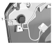
1. Turn bulb holder clockwise ti release it
