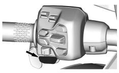
Press the button to activate the horn.
