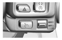
The button is used to activate the cruise control function
