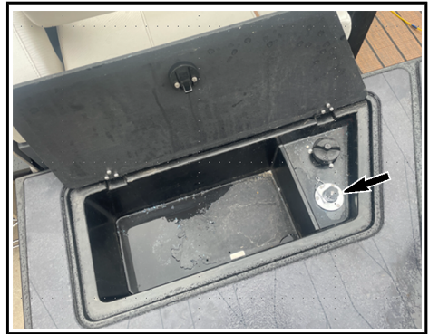
FLUSHING PORT — TYPICAL
