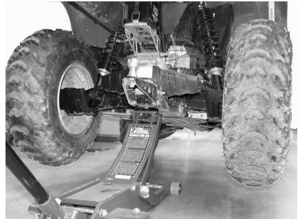
TYPICAL — REAR LIFTING POINT
