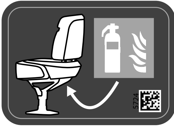
FIRE EXTINGUISHER POSITION LABEL
