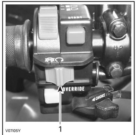
1. Engine stop switch
