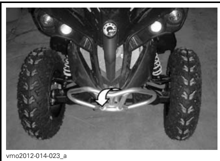
vmo2012-014-023_a TYPICAL - FRONT TIE-DOWN POINT LOCATION
