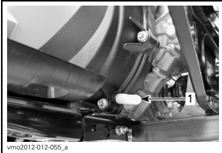
1. CVT drain reservoir
