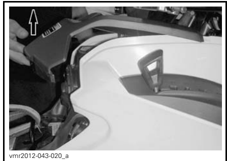
LIFT REAR PORTION
