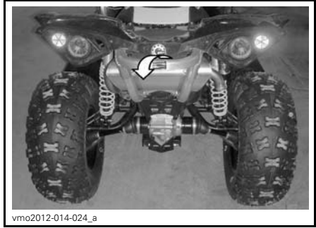
vmo2012-014-024_a TYPICAL - REAR TIE-DOWN POINT LOCATION
