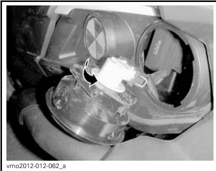
ROTATE BULB COUNTERCLOCKWISE
