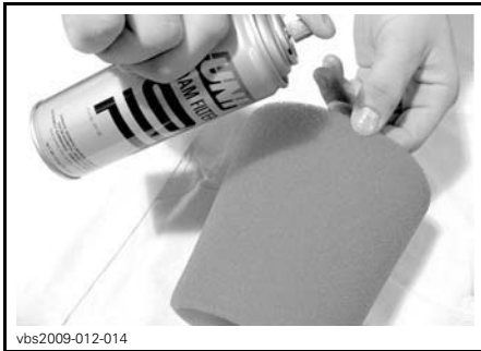
TYPICAL - OIL THE FOAM FILTER
