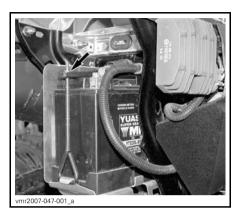
Pull out top bracket. Remove battery.
