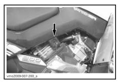
The lock purpose is to secure the transmission shifter lever in park position.
