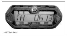
Press and HOLD display selection button for 2 seconds to reset the hour meter
