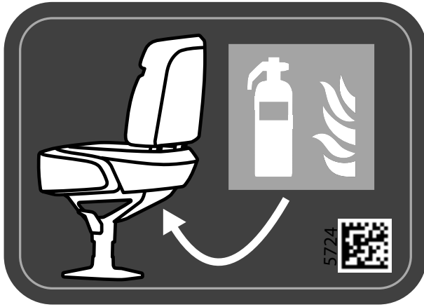
FIRE EXTINGUISHER POSITION LABEL
