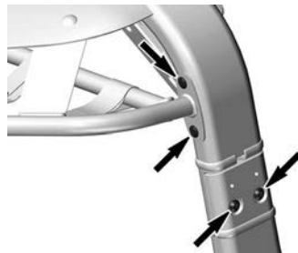
FRONT BIMINI STRUCTURE SCREWS – LH SIDE
