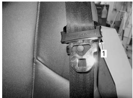
TYPICAL - LOCKED POSITION
