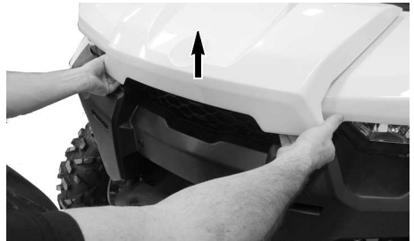
LIFTING FRONT SERVICE COVER EDGE.
