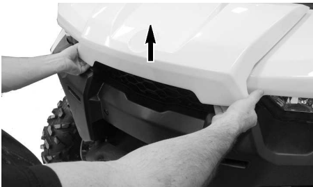
LIFTING FRONT SERVICE COVER EDGE.
