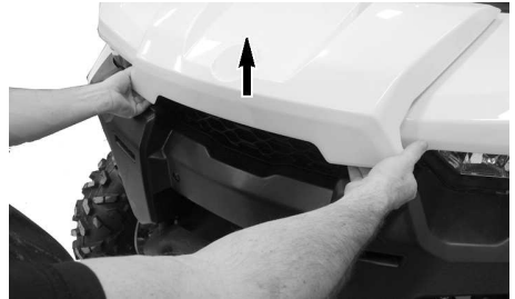
LIFTING FRONT SERVICE COVER EDGE.
