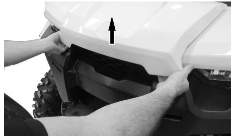
LIFTING FRONT SERVICE COVER EDGE.
