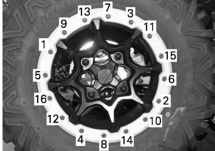
TYPICAL - TIGHTENING SEQUENCE
