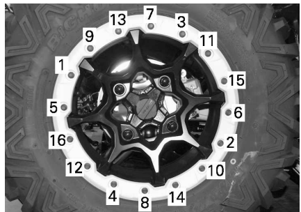
TYPICAL - TIGHTENING SEQUENCE
