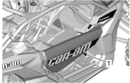
1. Door closed and locked in place
