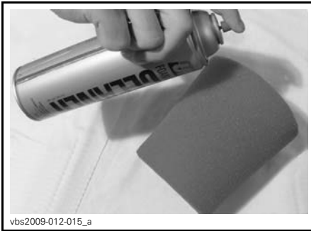
TYPICAL - SPRAY THE FOAM ELEMENT
