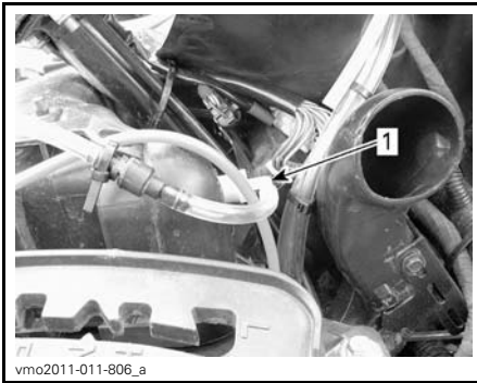
1. ACS compressor air filter inlet into air housing cover
