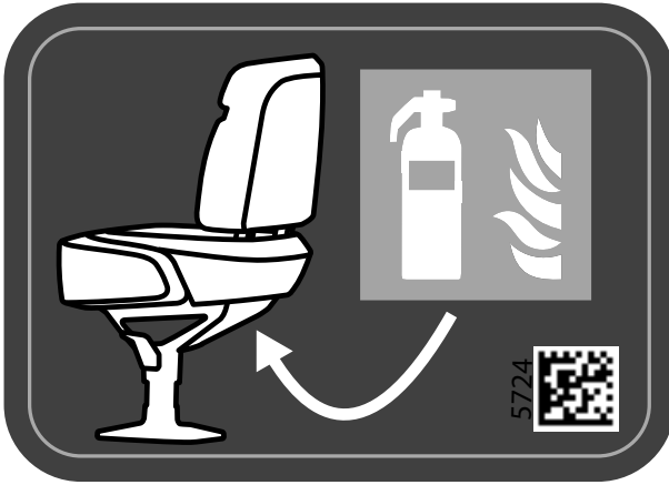
FIRE EXTINGUISHER POSITION LABEL
