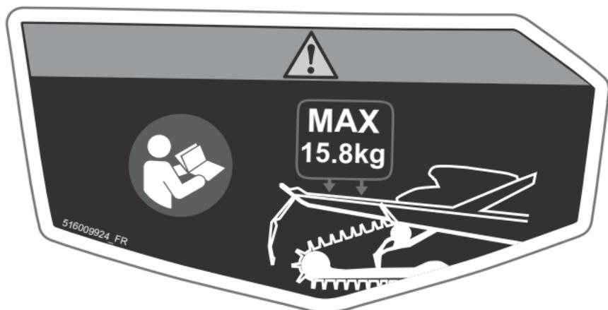
**CHARGE CARGO MAXIMALE ET CAPACITÉ DE REMORQUAGE - ÉTIQUETTE D'AVERTISSEMENT**
