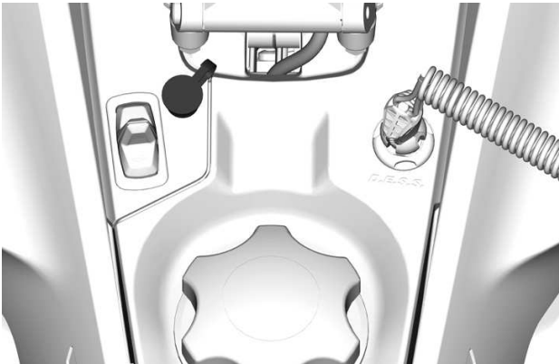
DRIVER - ELECTRIC VISOR JACK CONNECTOR LOCATION
